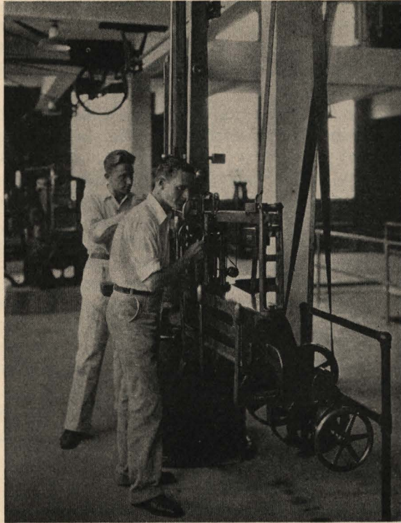
A tensile test on steel in college laboratory. The steel for all important uses must meet standard specifications of composition and physical properties.
